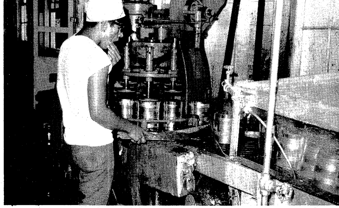
LIDS are automatically stamped on cans of cherries before cooking.
