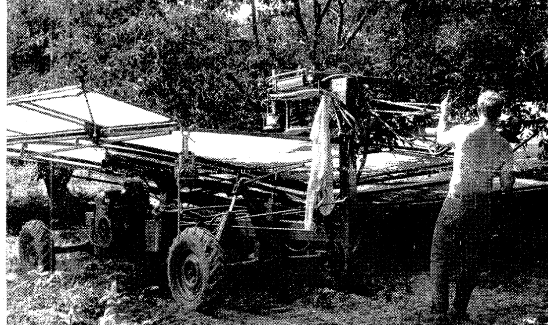
AN automatic cherry picker, termed a "shaker," and operated by Ted Sherman, can empty a tree in two minutes.
