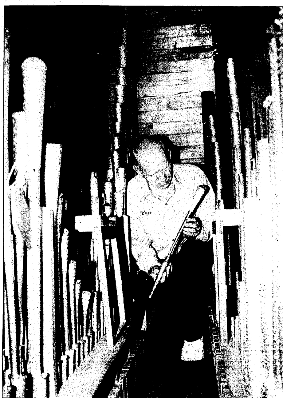
Pipe organ technician Roscoe Wheeler, pictured above in the back chamber of the pipe organ at Boyne City's United Methodist Church, along with his wife Carolyn, removed all 869 pipes of the organ and cleaned each one individually.
