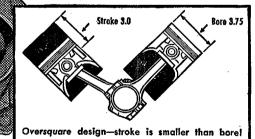
Here's the measure of a truly modern V8 engine-Chevrolet's advanced oversquare design. It means less friction . . . longer engine lifel
