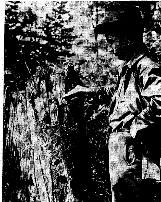
Gradually becoming a Michigan rarity are original bearing trees such as this one which Dean DeLaMater, conservation department surveyor, "discovered" near Gwin in a routine forest survey. Still partially visible but not entirely readable is the marking made in 1853, locating this particular spot as townline 44 north, range 25 and 26 west, linking sections 19, 24, 25 and 30. DeLaMater reports this is the first "location" tree he has come across in 12 years of forestry work. Tree was cut in early upper peninsula lumbering days. Most likely area to still find original bearing trees is in the few upper peninsula virgin timber tracts.
