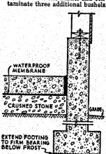
rier under the concrete. The strips are sealed at the edges.
