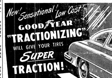
Tractionizing is the BEST method known to give tires extra grip on wet, slippery or icy roads. Tractionizing "tattoos" its thousands of rough-edged holes only into the top part of your original tough tread where it does the good . . . and does it right on your car.
