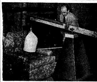
Wooden springs, wartime replacement for steel, are here being tested in the wood utilization laboratory of the University of Michigan for a Michigan manuacturer who is seeking O.P.A. approval. In this test, a 40-pound weight is tropped on the seat of a wooden-spring chair 10,000 times to see if it "can take Successful use of wooden springs, University technicians say, will save the jobs of many furniture workers and may reduce production costs in the furni-
