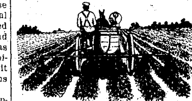
A Modern and Desirable Type of Potato Spraying Machine in Operation. —Will Spray 20 to 30 Acres Per Day. —Extra Nozzles Can Be Attached if Desired.—This Machine is Equipped with a Pump, Pressure Tank and Safety Valve.
